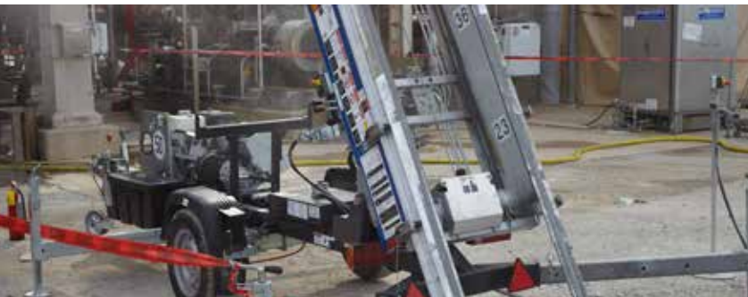
"The key is a basket at the end of the telescoping boom, able to lift 550 pounds of scaffolding up to 78 feet." ^
